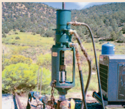
Oil field gas production is accomplished by using Rineer to drive the down hole progressive cavity water pump.
