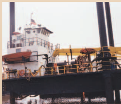
This Jack Up Boat uses nine Rineer motors per pile to stabilize the boat above water level to work on other equipment.
