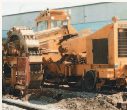
This Railroad Undercutter machine uses Rineer to power the ditching wheels and various conveyors.
