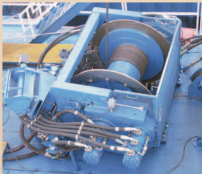
A large capacity winch is driven by two Rineer 250 CID motors plugged into the drum via a gearbox.
