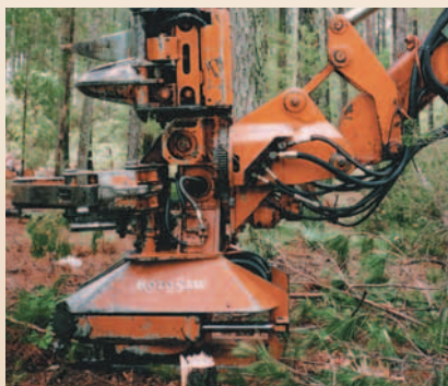
This Feller-Buncher uses Rineer to direct drive the large diameter saw blade.
