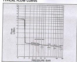
flow dividers are available in standard ranges 0 - 25 L/Min and 0 - 50 L/Min. Dimensions below show 0 - 25 L/Min unit.
