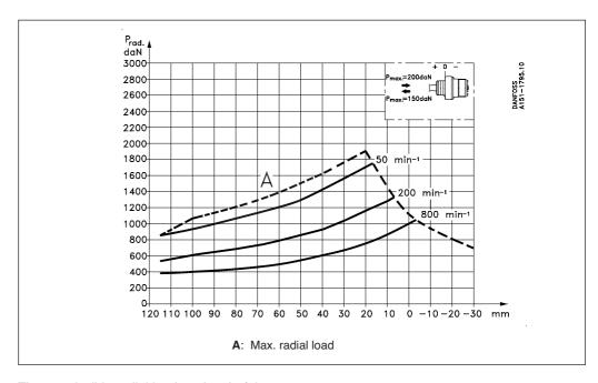
The permissible radial load on the shaft is shown for different speeds as a function of the distance from the mounting flange to the point of load application.
