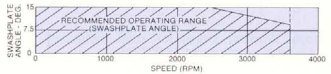
Swashplate Angle vs. Shaft Speed
