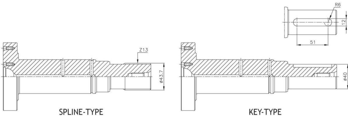
IT IS DIFFERENT ON THE SHAPE BETWEEN THE KEY TYPE AND SPLINE PLATE
